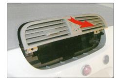
Remove the original Radio 1. and air vent cover
