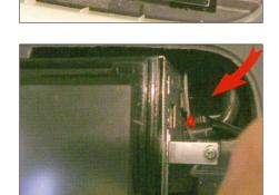
Insert the 2-DIN Navigation 6. into the cage until the springs click and engage fully
