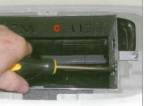
4. Locate the cage (C) in position, ensuring correct alignment to the foam block and fix it as shown
